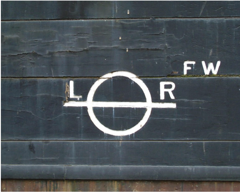
The Lloyd's Register load line marked on the hull of the Cutty Sark. Source: Wikipedia.
